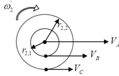
Figure 2. Velocities distribution on the compound gear 2
