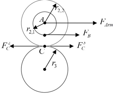
Figure 3. Forces distribution of compound gear 2
