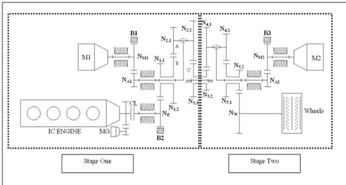
Figure1. Schematic diagram of hybrid vehicle transmission system
