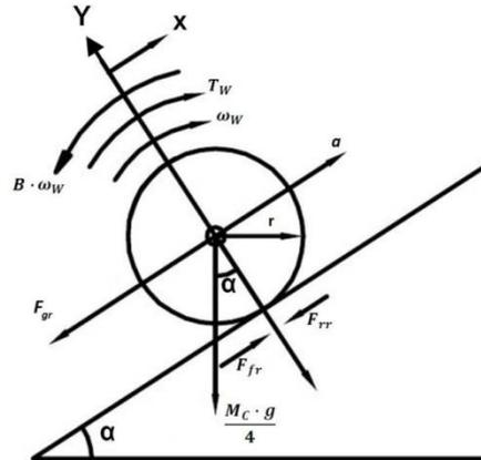
Figure 4. Vehicle single driving wheel on a ramp road
