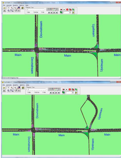
Figure 2. SimTraffic Snapshots Before and After Applying the RTS Design
