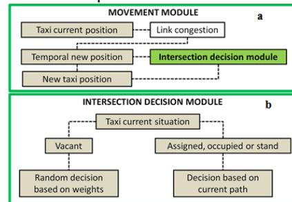
Figure 3. Movement (a) and Intersection decision (b) modules
